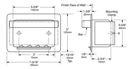
Rough Wall Opening 6" (150mm) wide 4" (100mm) high 4" (100mm) minimum recessed depth
